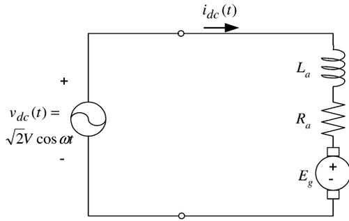
Fig. 2. Equivalent circuit of a dc drive during the turn-on period of a set of thyristors.
