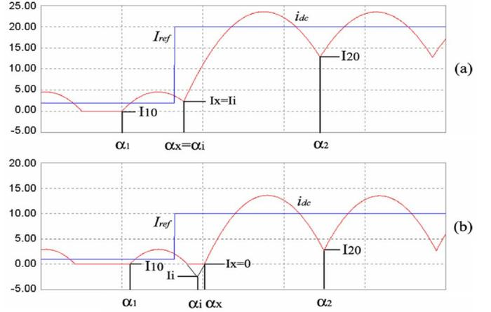
Fig. 5. Transition of the firing angle (a) with the intersection point above zero and (b) with the intersection point below zero.
