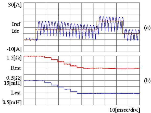
Fig. 15. (a) Current response by the controller parameter and (b) estimated  $R$ ,  $L$ .
