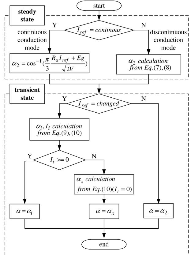
Fig. 6. Flow chart of firing angle calculation.
