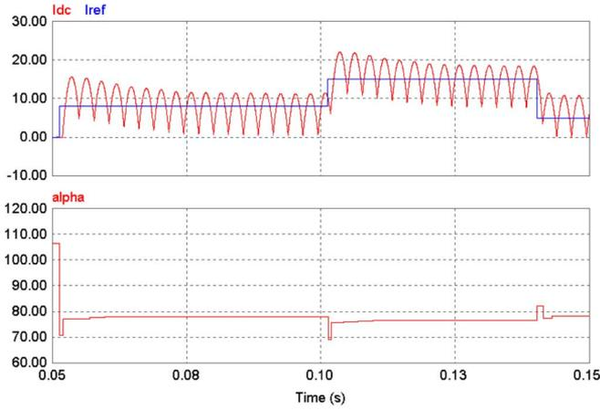
Fig. 10. Current control response and firing angle with a PI controller.
