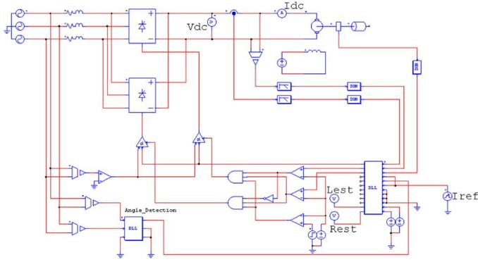
Fig. 7. Simulation circuit using a dc-motor load.
