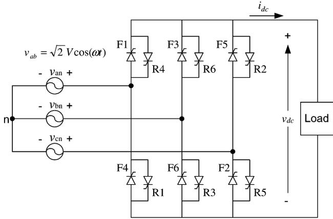
Fig. 1. Circuit of a dual thyristor converter with a dc load.
