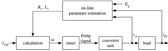
Fig. 4. Proposed predictive current controller with an online parameter estimator.
