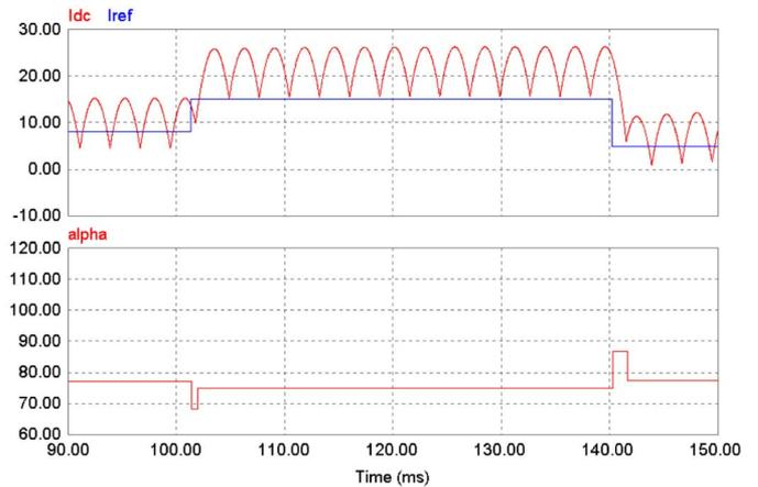
Fig. 9. Current control response and firing angle with 150% parameters.
