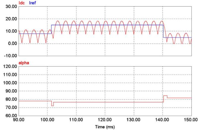
Fig. 8. Current control response and firing angle with 100% parameters.
