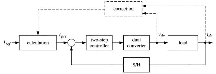
Fig. 3. Block diagram of a predictive controller.
