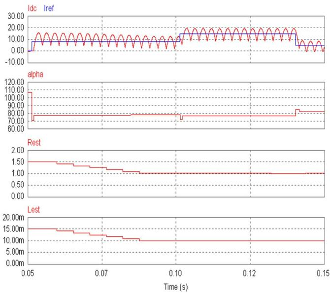
Fig. 11. Current control response, firing angle, and estimated  $R$  and  $L$  with the online parameter estimator.
