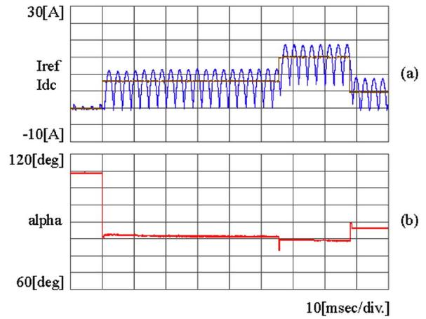
Fig. 13. (a) Current control response and (b) firing angle with 100% parameters.
