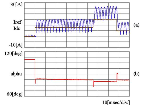
Fig. 14. (a) Current control response and (b) firing angle with 150% parameters.
